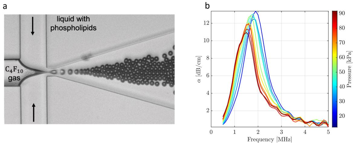
Figure 1, Image of the custom-made flow-focusing device used to produce  $C_4F_{10}$  filled monodisperse microbubbles. *b)* Acoustical characterization of phospholipid microbubbles suspended in water. The Y-axis shows the attenuation coefficient.
